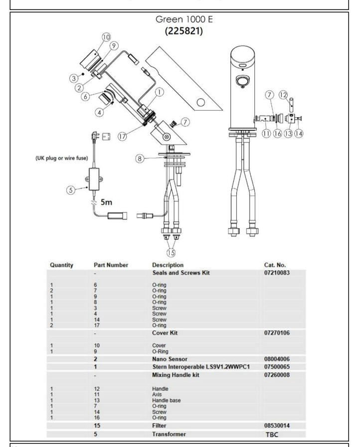
Note: In order to locate the relevant spare part, please check the corresponding parts and part mumber in the drawing. Minimum order quantity will be required.
